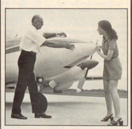
The Aztec E has a long, pointed nose with a recessed landing light. This model was built from 1971 through 1975.
