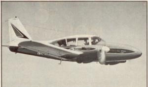
The Aztec B, built from 1962 through 1964, has six seats and a long, blunt nose that houses a forward baggage compartment.
