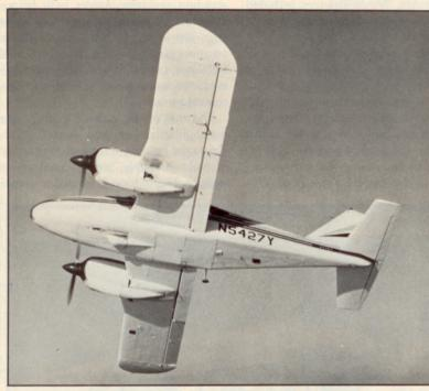
Slim engine nacelles and landing-gear doors differentiate the Aztec C from earlier models. The Aztec C was produced from 1964 through 1968. The D model, built in 1969 and 1970, looks very much like its predecessor but has ram's horn control yokes and rocker switches in the panel.
